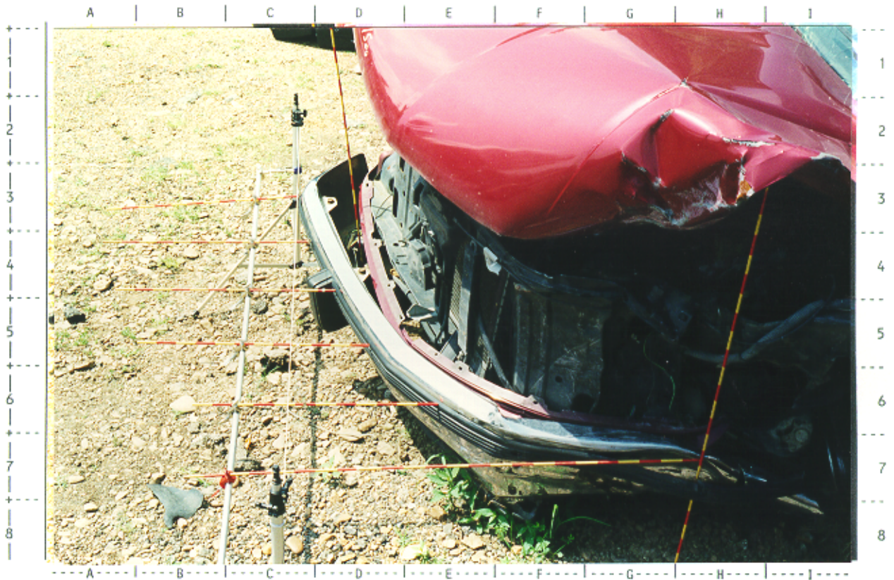
# 79 -- Front reference line viewed from L with contour gauge present shows damage to front left corner of '88 Chevrolet C-1500 pickup
